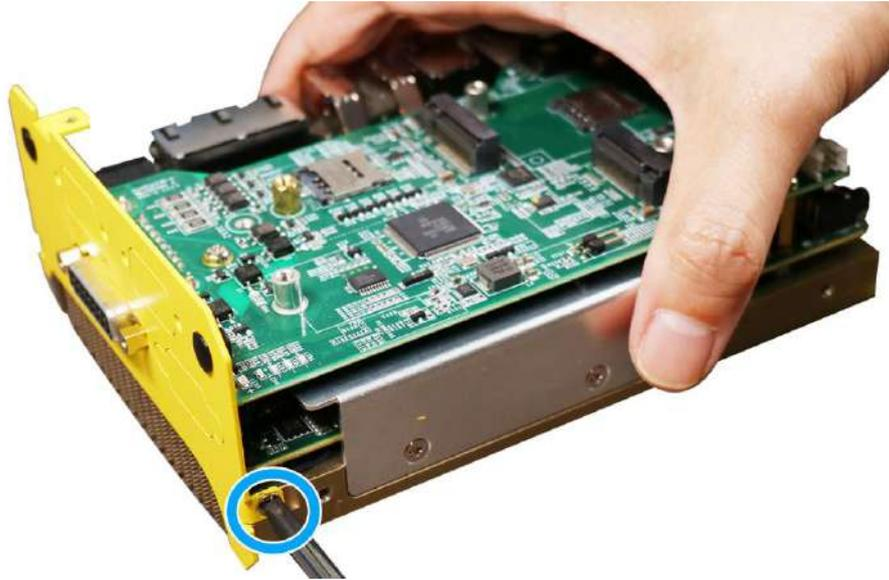
**Remove the screw securing the DIO panel**
