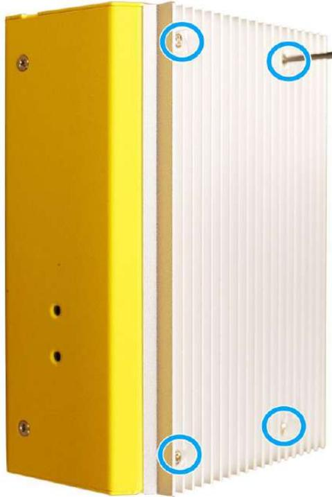
2. Gently lift the bottom heatsink off to access the M.2 B key slot on the MezIO™ card. Note the **copper standoff** can be adjusted to suit **2242/ 3042** or **3052** modules
