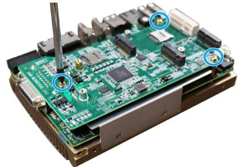
**Secure the MezIO™ module with the screws indicated**
