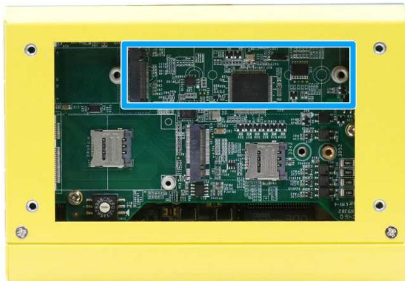
3. Insert the M.2 module on a 45 degree angle, press the module down and secure with a screw.
