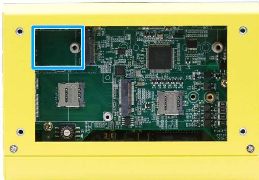
6. Insert the M.2 E key module on a 45 degree angle, press the module down and secure with a screw.
