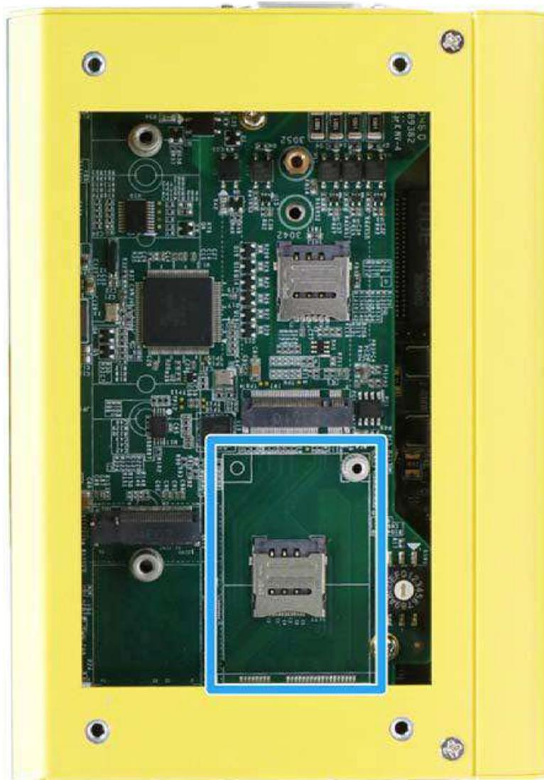
The system provides a mini-PCle socket (indicated in blue) for WiFi module installation. For WiFi wireless communication, multiple SMA antenna apertures can be located on the front and rear panel.
