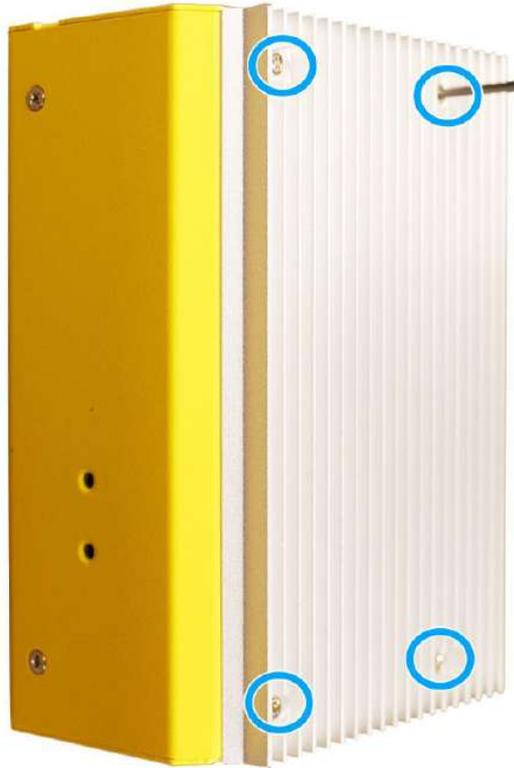
2. Gently lift the heatsink off to access the M.2 slot on the MezIO™ card.
