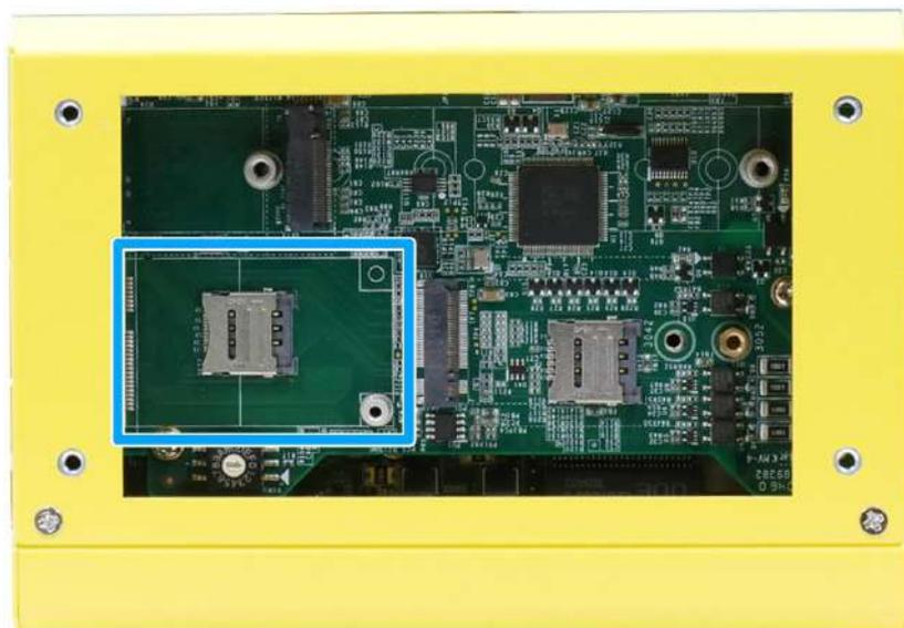
3. Insert the module on a 45 degree angle, gently press the module down and secure with a screw.
