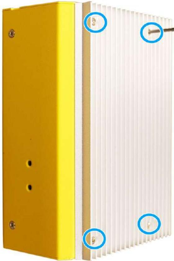
2. Gently lift the bottom heatsink to access the mini-PCIe slot.
