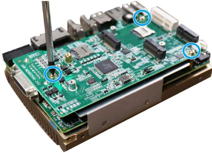
**Remove screws securing the MezIO™ module**
