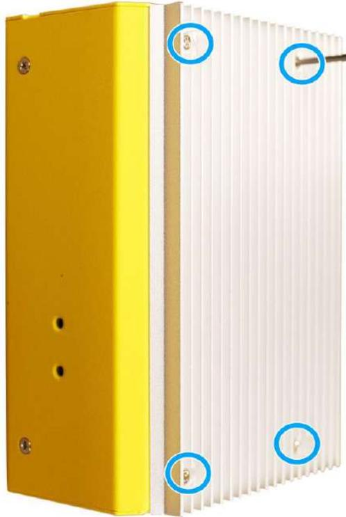
2. Gently lift the bottom heatsink off to access the M.2 E key slot on the MezIO™ card.
