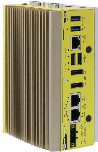
Connectivity-wise, POC-451VTC offers three 2.5GBASE-T Ethernet ports with PoE+ capability for powering PoE PD devices, such as IP and GigE cameras. The ports are backward-compatible with 1000/100 Mbps Ethernet to work with most existing Ethernet devices. The system also provides isolated DIO for sensor/ actuator control and 8V-35V wide range DC input with ignition power control for in-vehicle deployment.
