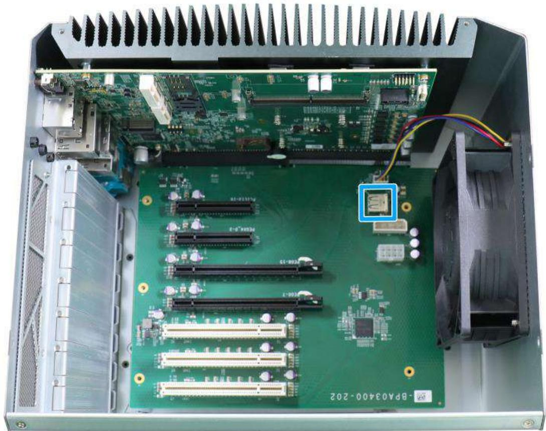
The system's daughter board has an internal USB2.0 port on the PCBA. You can utilize this USB port to connect a USB protection dongle inside the chassis of the system.
