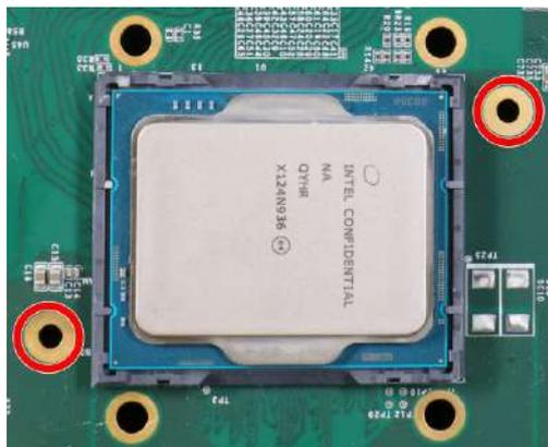
Screw holes for CPU retention bracket
