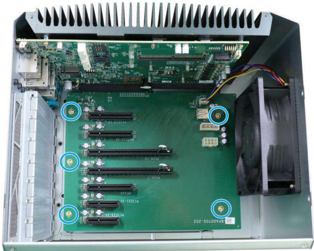
3. Disconnect the fan power cable and gently wiggle to disengage the daughterboard from the motherboard.
