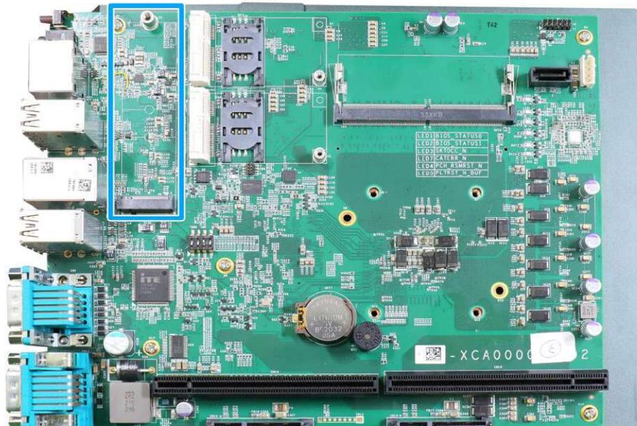
3. Insert the module on a 45 degree angle.
