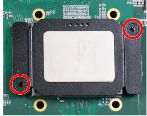
**Screw holes for CPU retention bracket**
