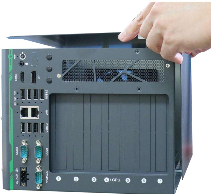
2. Secure the screw indicated on the I/O panel.
