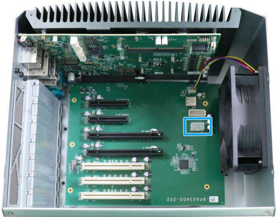
The system supports an NVIDIA graphics inference accelerator up to 115W. The 8-pin connector can supply additional power delivery to the graphics card for operation stability.
