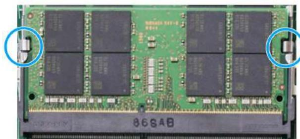
5. If you are installing the memory module on the CPU socket side, please remember to
