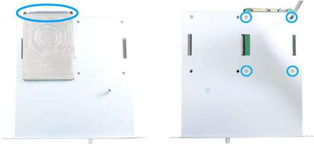
**SATA connectors facing inwards**      **Secure underneath with flathead screws**
