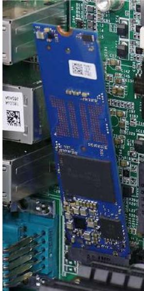
4. Gently press down and secure the module with an M3 P-head screw.
