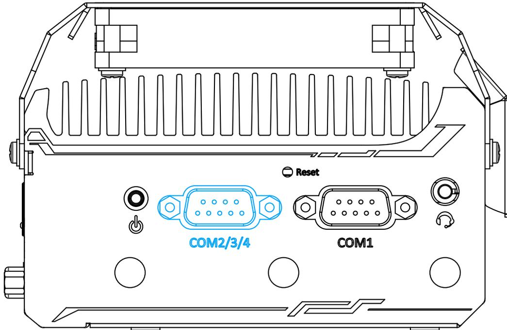
Implemented using industrial-grade ITE8786 Super IO chip (-40 to 85°C) and provide up to 921600 bps baud rate, the D-Sub male connector (COM2/ 3/ 4) can be configured in the BIOS as single RS-422/ 485 port (COM2) or three 3-wire RS-232 ports (COM2/COM3/COM4). Please refer to [COM2/ 3/ 4 Port Configuration](#) for configuring operation mode. An optional 1-to-3 Y-cable is available to connect three RS-232 devices.
