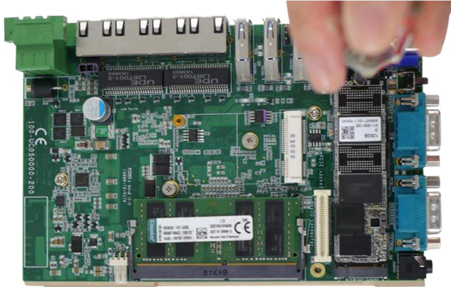
5. Once you have installed the NVMe SSD, you need to reinstall the heat spreader but before you do so, please make sure the protective film on the thermal pads have been removed.
