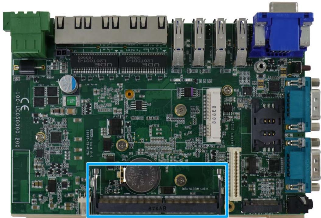
The system supports one 260-pin SO-DIMM socket for installing DDR4 memory module up to 16GB in capacity. Please refer to the following table for details.
