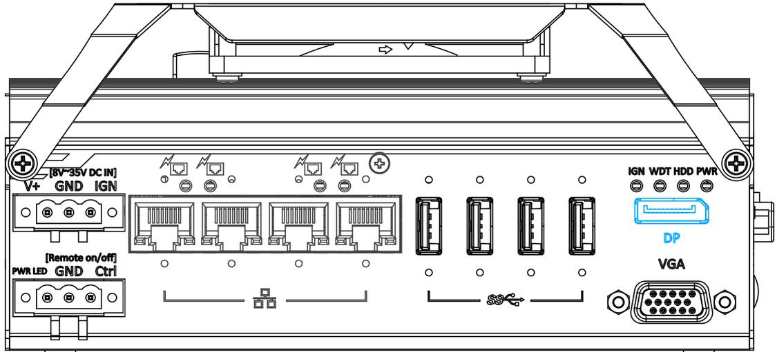
The system has a DisplayPort (DP) output which is a digital display interface that mainly connect video source and carry audio to a display device. When connecting a DP, it can deliver up to 4K UHD (4096 x 2160 @ 30Hz) in resolution. The system is designed to support passive DP adapter/ cable. You can connect to other display devices using DP-to-HDMI cable or DP-to-DVI cable.
