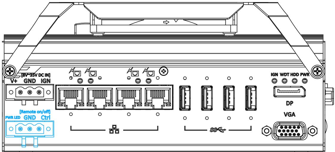
The “Remote On/ Off” 3-pin connection allows for external switch extension. It is useful when the system is placed in a cabinet or a not easily accessed location. You may connect an external remote with an external status LED indicator (15mA) by connecting to PWR LED and GND.
