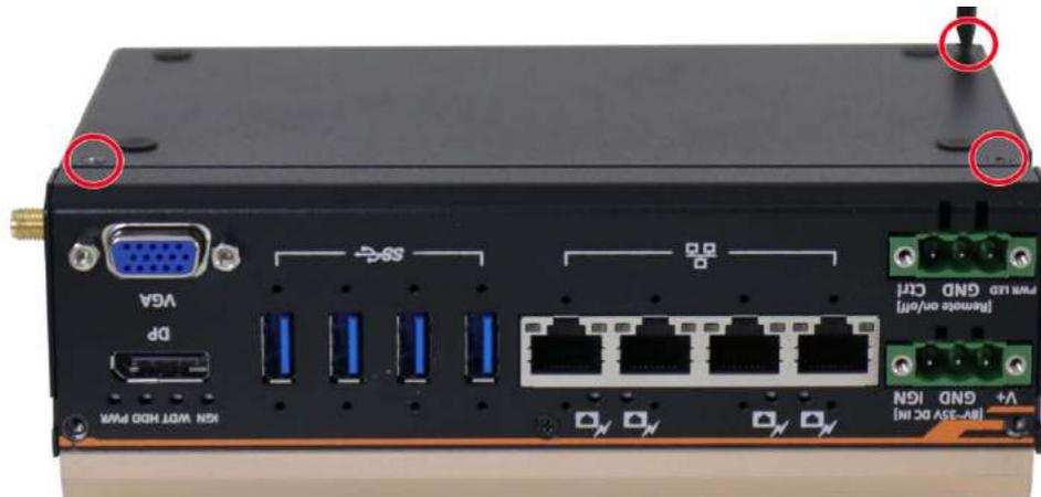
6. Unscrew the two (2) VGA hexa bolt screws (indicated in red); unscrew the three (3) screws (indicated in blue) and gently remove the front I/O panel.
