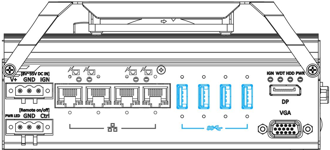
The system offers four USB 3.1 Gen1 (SuperSpeed USB) ports on its front panel. They are backward compatible with USB 2.0, USB 1.1 and USB 1.0 devices. Legacy USB support is also provided so you can use USB keyboard/mouse in DOS environment while USB 3.1 Gen1 driver is supported natively in Windows 10.
