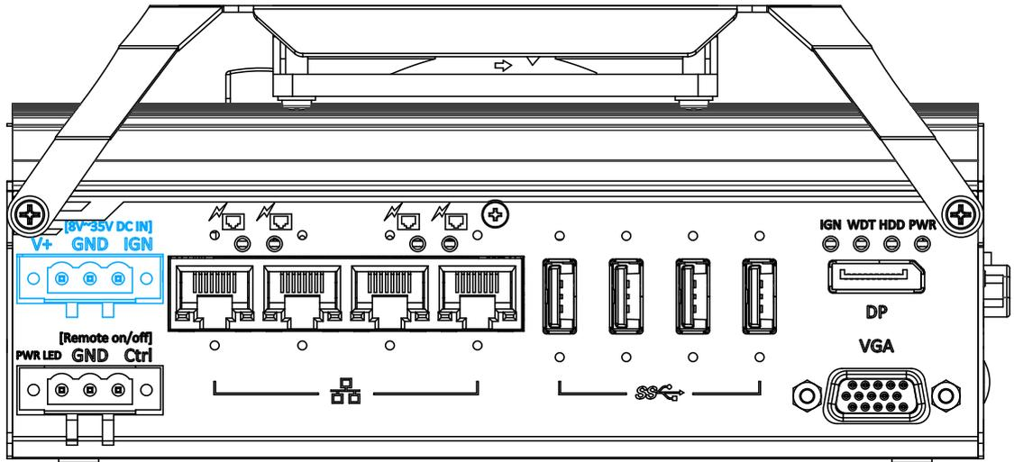
The system accepts a wide range of DC power input from 8 to 35V via a 3-pin pluggable terminal block, which is fit for field usage where DC power is usually provided. The screw clamping mechanism on the terminal block offers connection reliability when wiring DC power.
