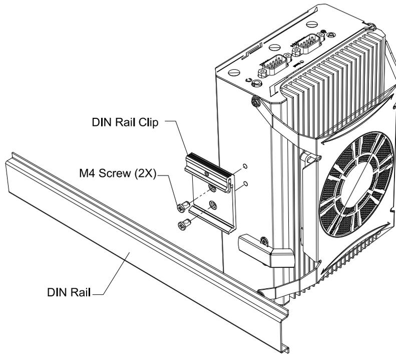
2. To install the DIN rail clip onto the DIN rail, you must come over the top of the DIN rail, tilting, overlap the top clip edge of the DIN rail clip onto the DIN rail first, and then firmly press the bottom-front of the enclosure to clip the bottom edge of the mount plate.
