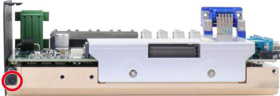
2. Install the front panel by securing it with three (3) screws (indicated in blue and green) and the two (2) hexa bolt (indicated in red) on the VGA connector. For POC-545/ 546 systems, please place the fan beneath the heatsink and secure it with screws (indicated in green).
