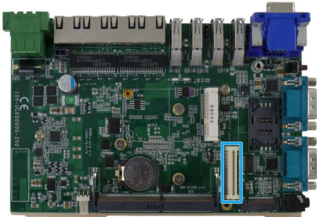
MezIO™ is an innovative interface designed for integrating application-oriented I/O functions into an embedded system. It offers computer signals, power rails and control signals via a high-speed connector. MezIO™ is also mechanically reliable benefited from its 3-point mounted mezzanine structure. A MezIO™ module can leverage these signals to implement comprehensive I/O functions.
