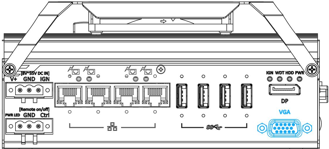
VGA connector is the most common video display connection. The VGA output supports up to 1920x1200@60Hz resolution.
