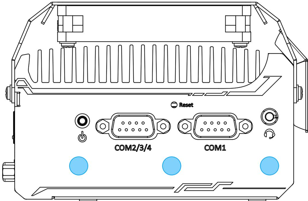
The system offers three SMA antenna openings reserved for SMA antenna installations. Users can take advantage of these three openings when installing mini-PCIe module for wireless communication reception such as 3G, 4G, GPS or WiFi.
