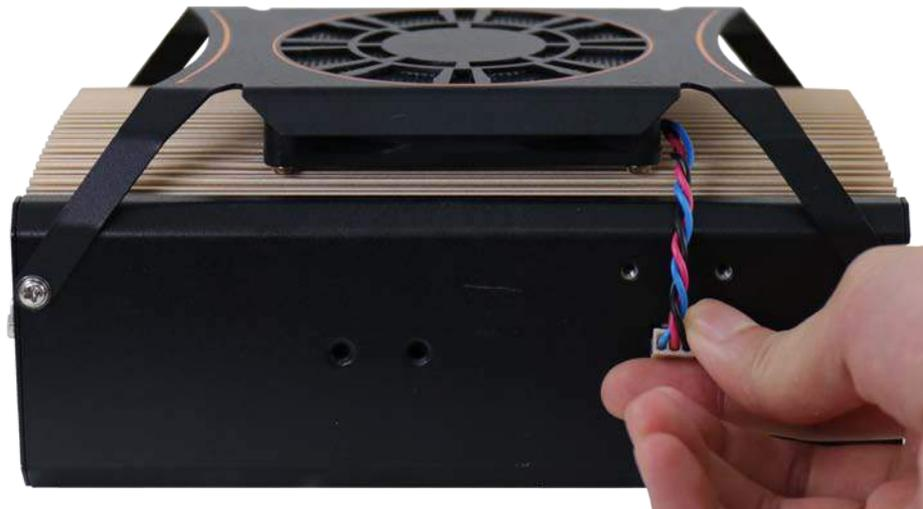
4. Remove the two (2) screws (indicated in red). For POC-545/ 546 systems, please also separate the fan from the enclosure.
