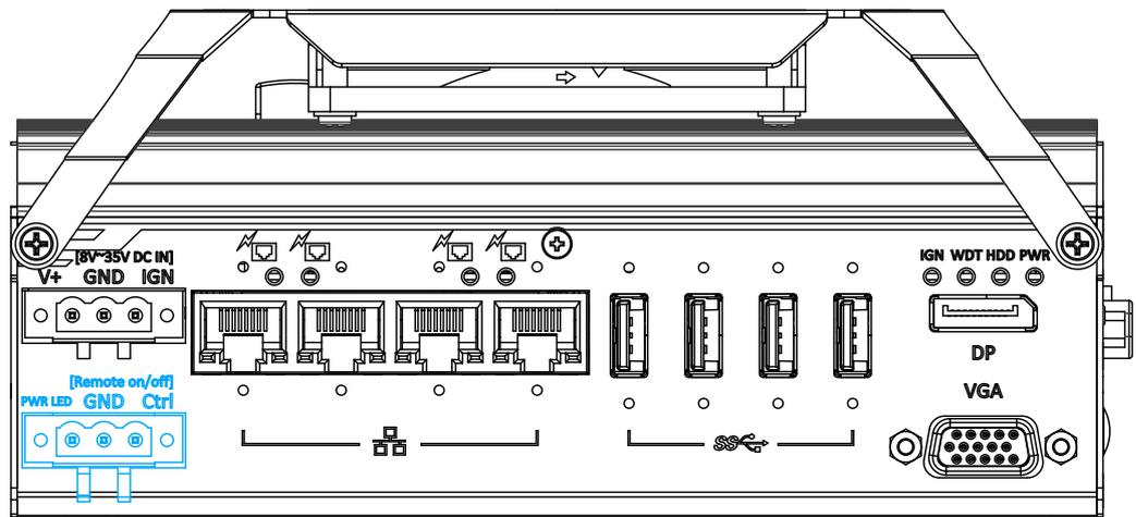
3. With DC power connected, pushing the power button will turn on the system and the PWR LED indicator will light up. Pushing the button when system is on will turn off the system. If your operating system supports ATX power mode (i.e. Microsoft Windows or Linux), pushing the power button while the system is in operation will result in a pre-defined system behavior, such as shutdown or hibernation.
