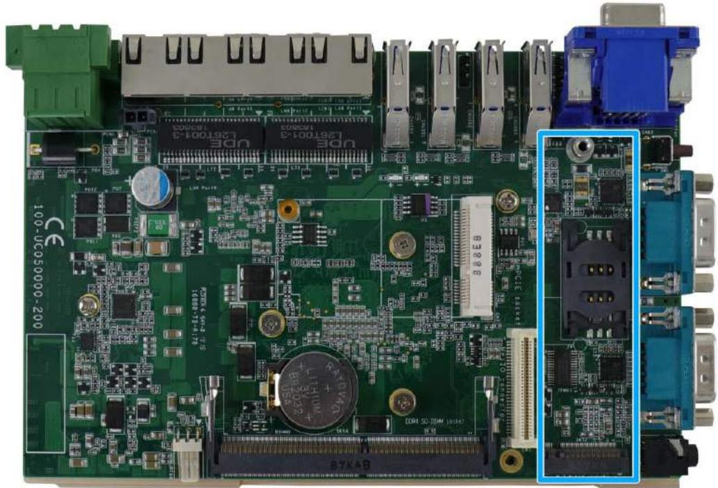
The system has an M.2 2280 slot (M key PCIe Gen3 x2) to install an NVMe SSD for the ultimate disk read/ write performance. An NVMe SSD offers doubled the disk read/ write speed performances over 2.5" SSDs.
