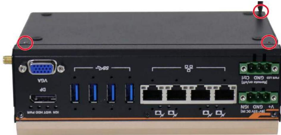
10. Secure the two (2) screws (indicated in red) to complete the enclosure assembly for POC-515/ 516 systems. For POC-545/ 546 systems, please secure the fan onto the enclosure.
