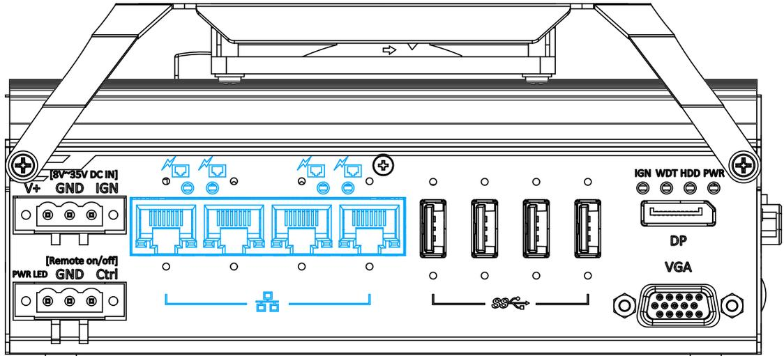
The Gigabit Power over Ethernet (PoE) port supply power and data on a standard CAT-5/CAT-6 Ethernet cable. Acting as a PSE (Power Sourcing Equipment), compliant with IEEE 802.3at, each port delivers up to 25W to a Powered Device (PD). PoE automatically detects and determine if the connected device is PoE PD or not before supplying power, making it compatible with standard Ethernet devices as well.
