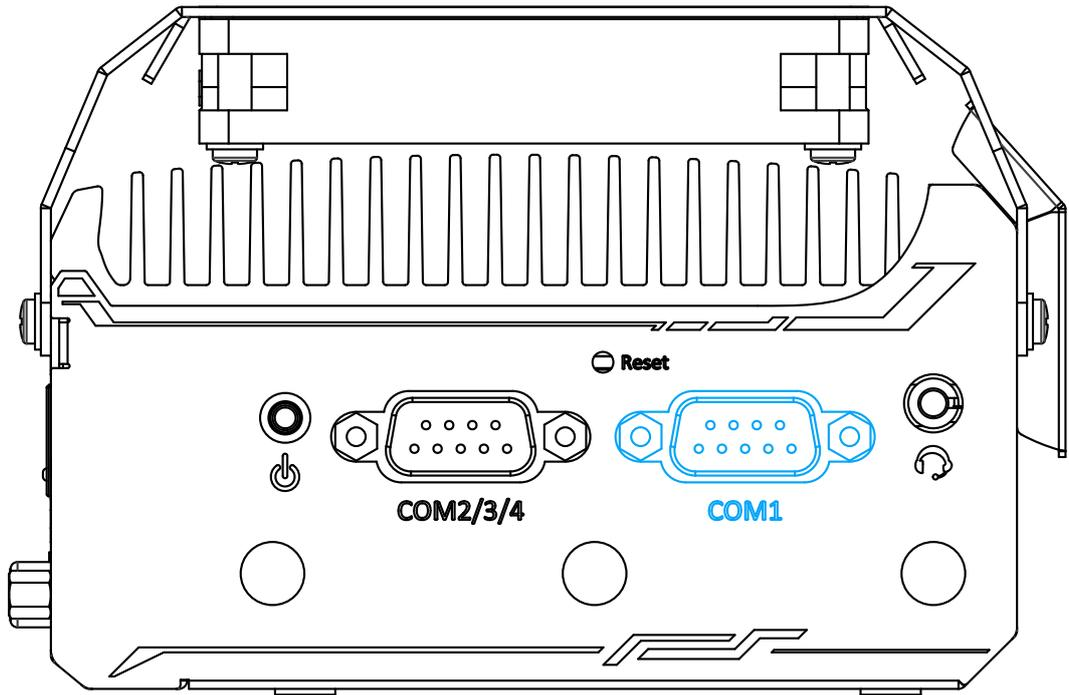
Implemented using industrial-grade ITE8786 Super IO chip (-40 to 85°C) and provide up to 921600 bps baud rate, COM1 is a software-configurable RS-232/422/485 port via 9-pin D-Sub male connector. The operation mode, slew rate and termination of COM1 can be set in BIOS setup utility. The following table describes the pin definition of COM ports.
