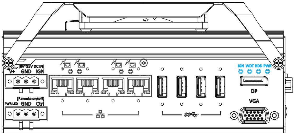
There are four LED indicators on the front panel: IGN, WDT, HDD and PWR. The descriptions of these four LEDs are listed in the following table.
