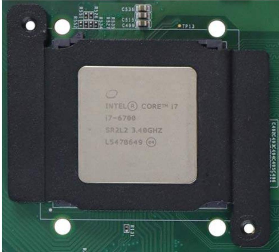
4. Turn the motherboard around and secure the bracket by tightening two M3 P-head screws.
