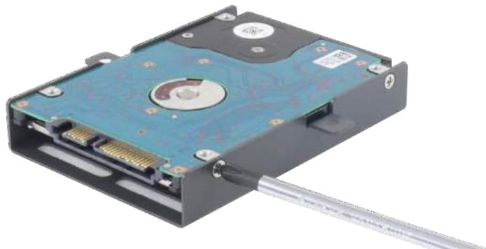
3. Gently insert the SATA port of HDD/ SSD to SATA port 1, the two screw hole should meet the standoffs on the motherboard, screw using two M3 P-head screws.
