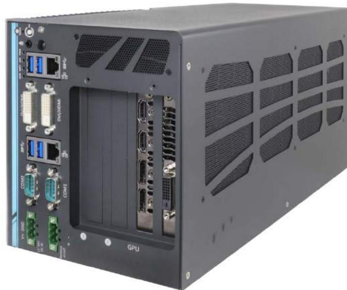
In order to sustain high GPU performance in industrial environments, Nuvo-6108GC features patented cold air intake design to effectively dissipate heat generated by the graphics card. The unique design guarantees operation at 60°C with 100% GPU loading and ensures Nuvo-6108GC's reliability for demanding field use. In addition, Nuvo-6108GC comes with patented shock/ vibration absorption mounting brackets to ensure the system's smooth operation under harsh environments.
