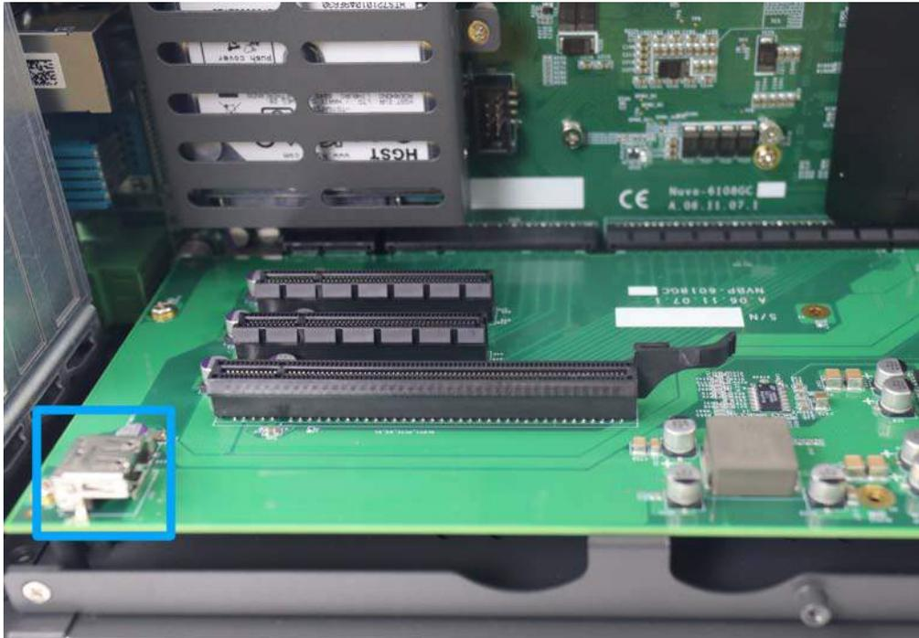
The system's daughter board has an internal USB2.0 port on the PCBA. You can utilize this USB port to connect a USB protection dongle inside the chassis of the system.
