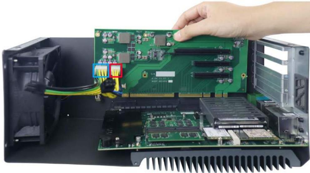
For high performance graphics cards, an additional 12V input is required. The system offers an 8-pin and a 6-pin PCIe power connector on its daughter board. It supports a PCI Express graphics card with up to 250W TDP.
