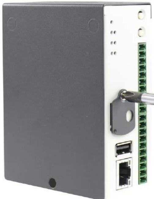
3. Place your thumbs firmly on the side of the enclosure and gently push upwards to remove the cover.
