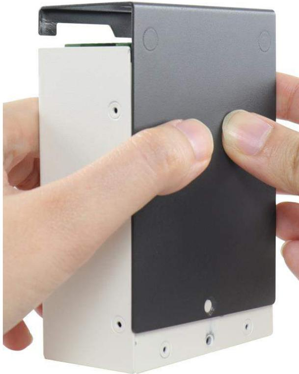
4. Once you have removed the cover, unfasten two screws that secure the PCBA in the enclosure.
